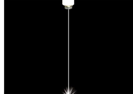
GDA needle jet nozzles are a one-piece construction, suitable to work with operating pressures lower than 20 bar and have a hard ruby spray tip, ideal to work with pressures lower than 200 bar. They are precisely machined and have a hydrodynamic design to produce a solid stream needle jet. Their stainless steel body and ruby tip ensure a long service life and a high resistance to wear.
